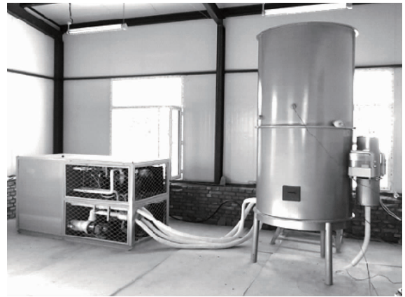
图1 1200 L等温云室外观 Fig.1 The external view of 1200 L isothermal cloud chamber
